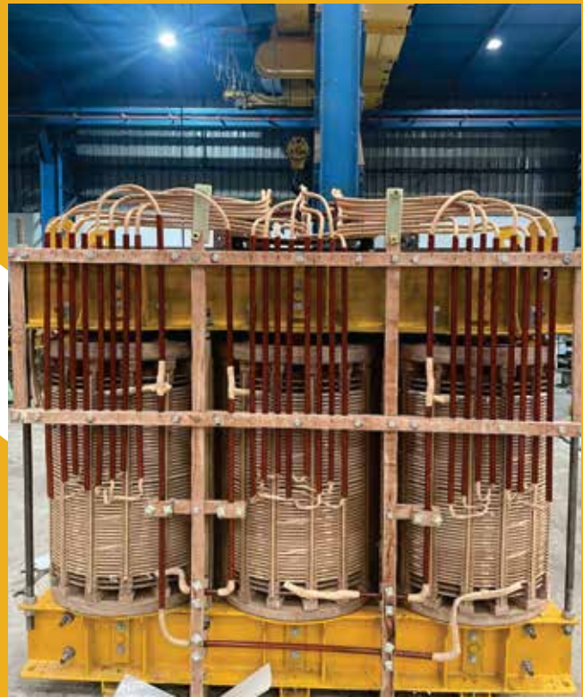
ACTIVE PART OF 4.5MVA 33000/433V ROLLING MILL DUTY TRANSFORMER OF SIGMA GROUP, KANPUR, U.P
